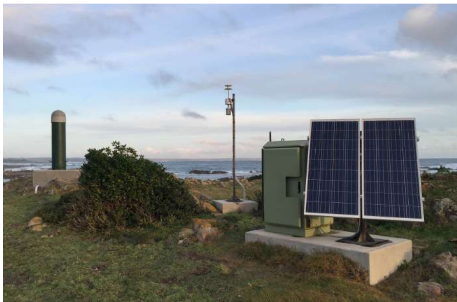
Image: GNSS ground station on King Island, Tasmania
