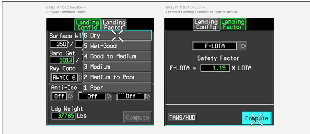
Figure 3. Honeywell MCDU with braking action, associated RWYCC and landing distance factor
